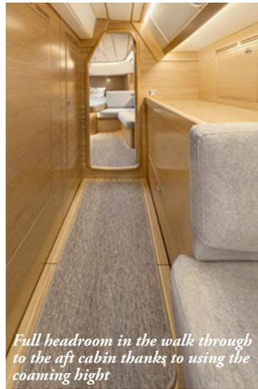
*Full headroom in the walk through to the aft cabin thanks to using the coaming height*
